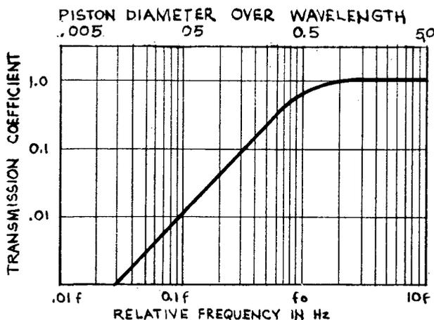
Fig. 1. Transmission coefficient versus frequency for circular piston in very large flat baffle.
